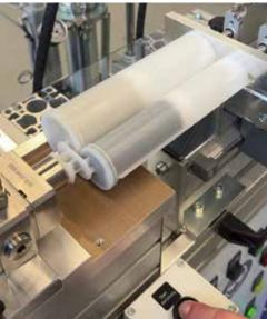
Automatically switches off when cartridge fill level is reached
