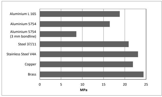
Note: Araldite® 2053 is not suitable to bond galvanized steel, for this type of substrate the Araldite® 2047-1 or the Araldite® 2051 may be used.
