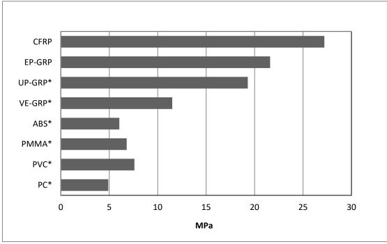
(\*): UP-GRP, VE-GRP, ABS, PMMA, PVC, PC, substrate's failure or substrate's delamination failure observed.
