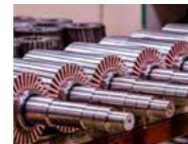
Bonding of sheet metal packages, commutators and bearings
