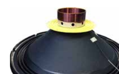
Project: Bonding of damping with voice coil and membrane
