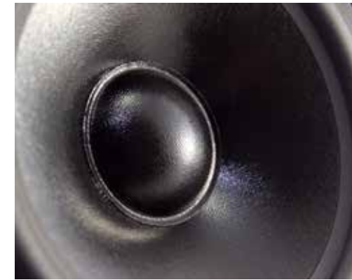
Bonding of dust cap with membrane
