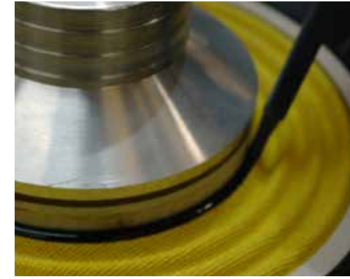
Bonding of damping with voice coil
