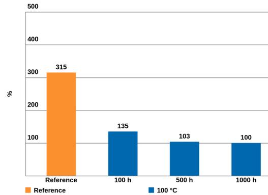
Compression shear strength after temperature storage
